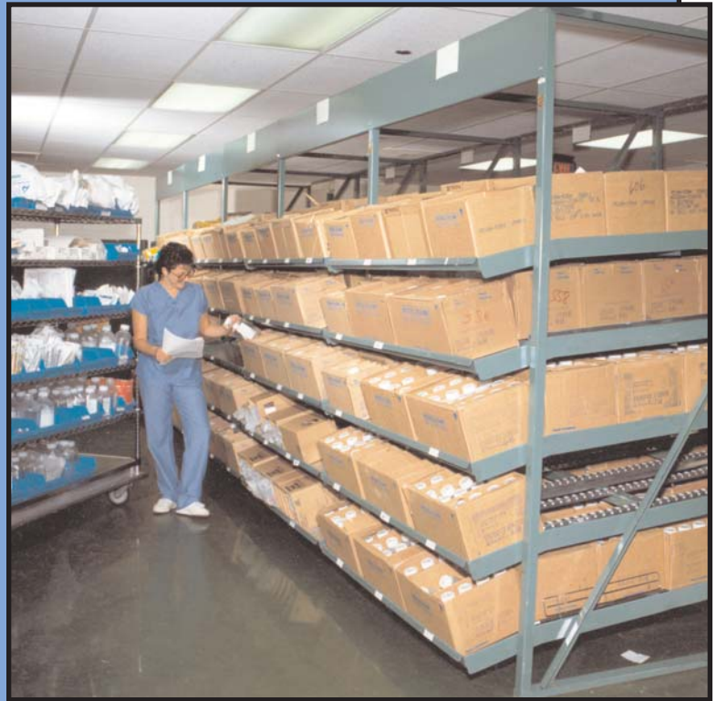
Items are selected from gravity flow rack and placed on carts for distribution to pharmacy, nursing, abulatory care units, etc...
